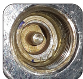
Example of a damaged seal
