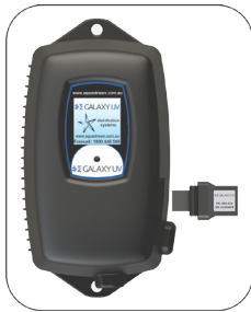
Figure 8. Lamp Key Installation
